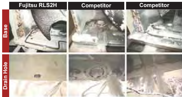
Drain hole is not filled, no freezing of base | Freezing where there is no heater | Drain hole is closed, large freezing of base
